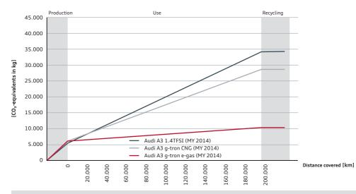
The additional expenditures especially due to the use of fiber-reinforced plastics in the gas tanks are already amortized at just over 5,000 km (Audi e-gas) or within the first 22,000 km (fossil fuel-derived natural gas).
