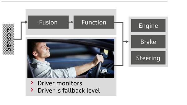
In critical situations, immediate driver reaction is required
