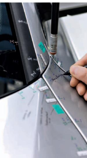
Audi vehicles are measured, described and evaluated both inside and out on the master jig. Any deviations are recorded on the car. The objective is to coordinate all components, gaps and flush alignments precisely with one another.
