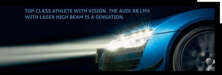
For each headlight a laser module made up of four laser diodes creates a blueish cone of light. A phosphorus converter transforms this cone into white light. This boosts the illumination range and sharpens contrast thanks to a wavelength of 450 nanometers and a color temperature of 5,500 kelvin.
