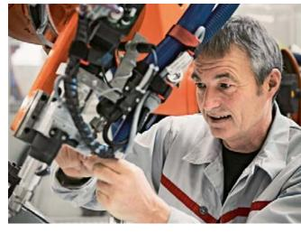
Industrial mechanic Peter-Michael Hahn inspects the filling valve on a gluing robot to ensure correct dosage.
