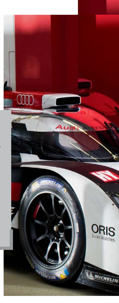
The **Le Mans Audi R18 e-tron quattro racing car** also features hybrid drive – in a very special form. A V6 TDI delivers almost 400 kW (approximately 540 hp) of power to the rear wheels. An electric motor, driven by a flywheel system, propels the front wheels with more than 170 kW for a few seconds at a time. In winning the 24 Hours of Le Mans in 2014, the hybrid racing model used 22 percent less fuel than its predecessor with conventional drive.
