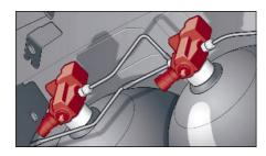
► Each gas tank is equipped with its individual cylinder valve and manual stopcock.
