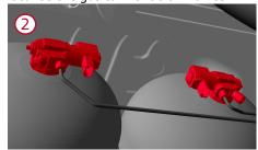
Turn the shut-off valve clockwise to the stop with a size 5 open-jaw or ring spanner
