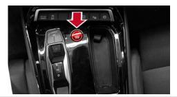
Press the START-STOP button without depressing the brake pedal
