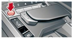
Press the START-STOP button without operating the brake pedal.
